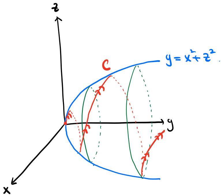
Note  $x = t \cos t$  and  $z = t \sin t$  together yield a rotation around the  $y$ -axis with increasing radius, while  $y = t^2$  moves to the positive  $y$ -direction.
