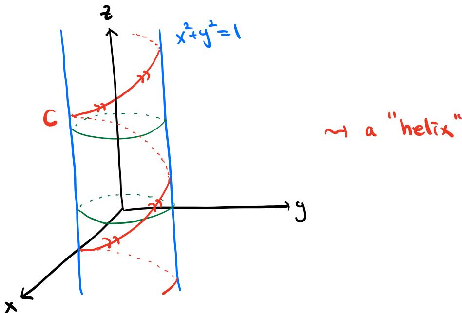
Note  $x = \cos t$  and  $y = \sin t$  together yield a rotation around the  $z$ -axis, while  $z = t$  moves upward.
